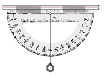
Using scotch tape, carefully attach the plastic straw to the straight edge of the protractor. Be sure that the string is not caught in the tape. The string needs to move freely.
